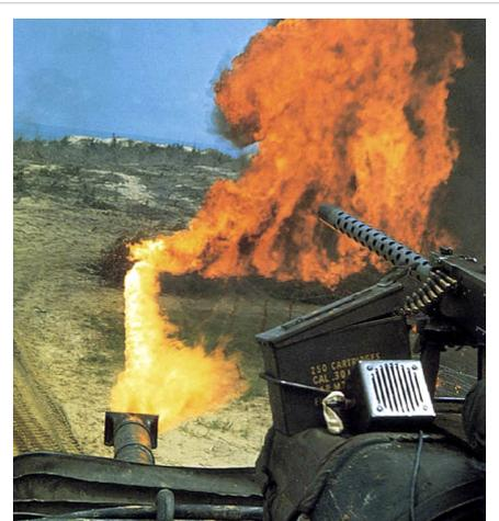
View from the turret of an M67 "Zippo". On the right is a mounted M1919 Browning machine gun with an attached box of linked .30-06 ammunition.
