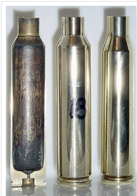
From left to right: cross sectioned and normal .338 Yogi cartridge cases compared to a factory .338 Lapua Magnum case.
