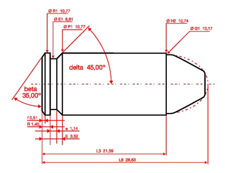
.40 S&W maximum C.I.P. cartridge dimensions.<sup>[]</sup> All sizes in millimeters (mm).
