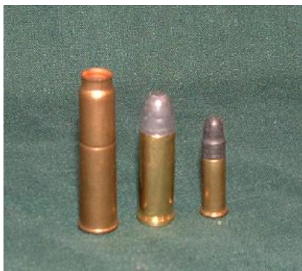
7.62×38R (7.62 Nagant) cartridge ( left ), shown next to a .32 S&W Long Cartridge and a .22 LR cartridge for comparison.
