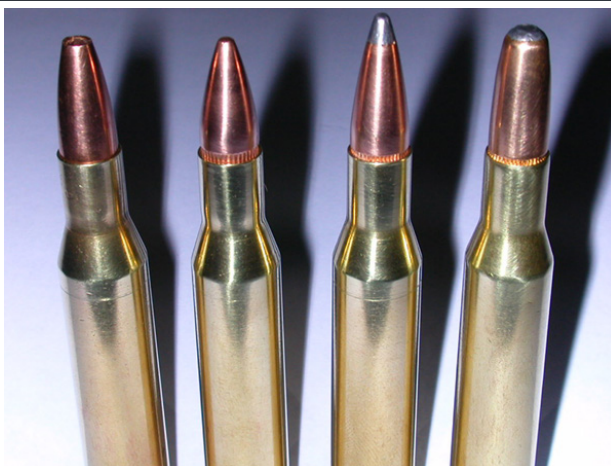
Left to Right 130-grain (8.4 g) - Hollow Point, 100-grain (6.5 g) FMJBT, 130-grain (8.4 g) Soft point, 160-grain (10 g) round nose.
