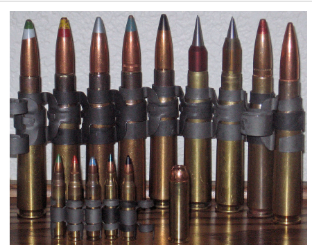
Left to right, rear: Mk211, Spotter, Silver tip (Armor Piercing Incendiary), Blue tip (Incendiary), Black tip (Armor Piercing), SLAP-T, SLAP, Tracer, and Ball. Front row are 5.56×45mm NATO and .500 S&W Magnum for size comparison.
